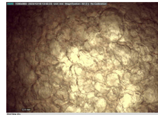
Figure 11. Biofoam after two wetting and drying processes
