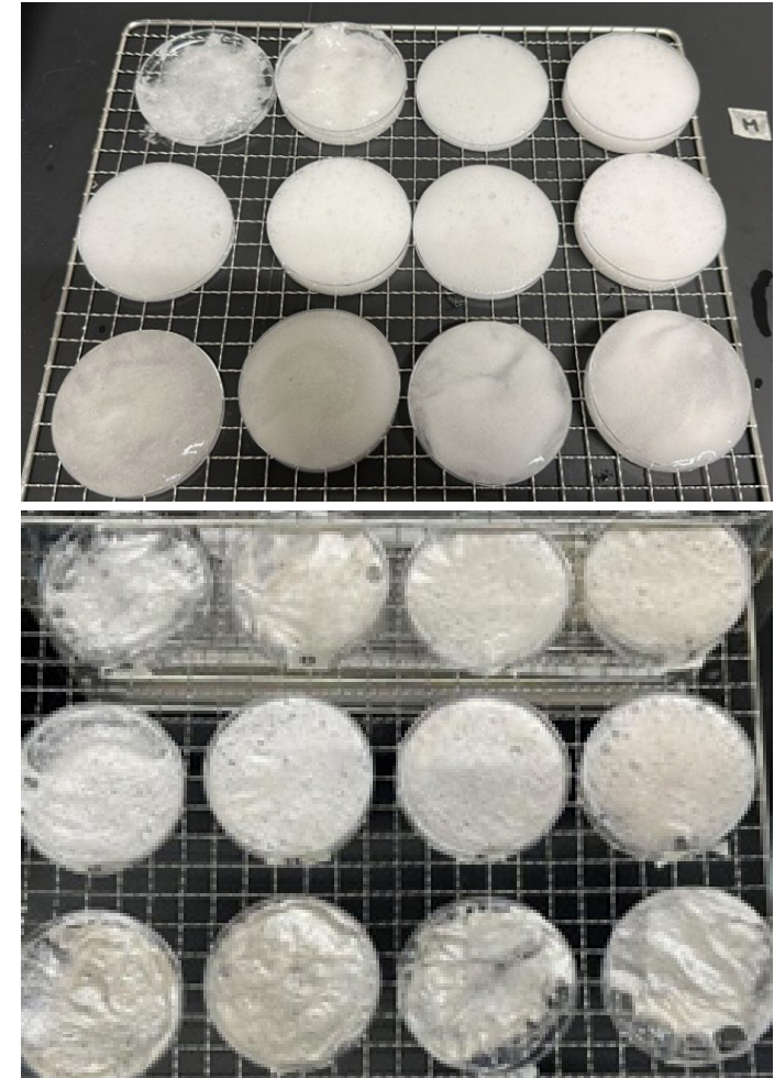
Figure 7. Konjac foam with different proportion, before (up) and after drying (down).
