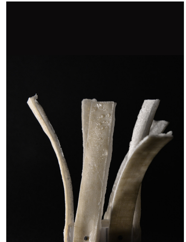
Figure 1. The imitation of flower blooming using the shape changing biofoam
