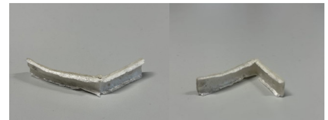
Figure 14. Bend the final material sample in two directions, towards the linen layer (left) and towards the foam layer (right).
